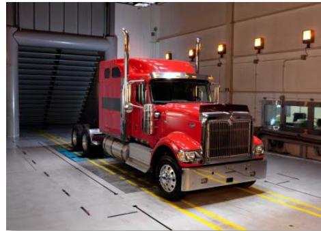
The “vehicle” test lab is also used for non-vehicle applications (generators, roof top HVAC&R units, study impact of wind on test article, cold start testing, etc.).
